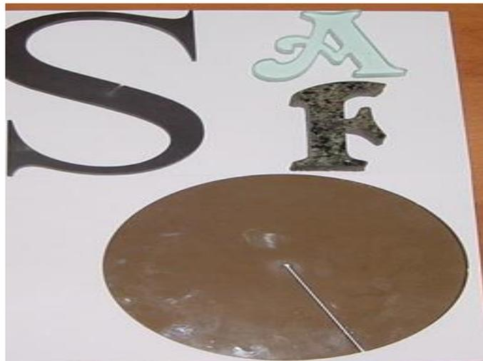
Fig.3. Laser cut examples of technology (glass, composite, stone, sital)
